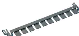
LSA 2/10-ES (Art.No. 24 01 33) Pluggable grounding rail: For 10DA connection modules serving as connection between LSA backmount frame and 1 DA surge voltage (+surge current) protection connector Installation: Plug into front connection modules, bonding to ground via LSA backmount frame
